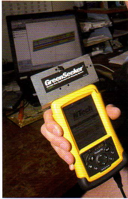
The GreenSeeker can map N levels across a paddock and, when combined with GPS and variable rate technology, can vary nitrogen applications "on the go" on the basis of the crop's NDVI.
