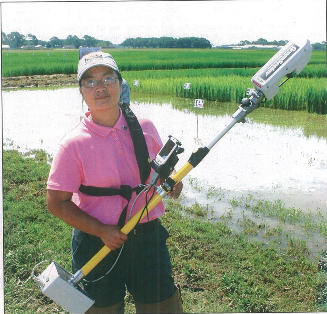
HAVING SETTLED ON the GreenSeeker technology for her rice and sugarcane studies, Brenda Tubana, LSU AgCenter assistant professor, is now busy taking readings and building a database. The readings will be used to establish the equation for crop yield potential. In turn, that information will help estimate, or project, the nitrogen requirements of the crop.
