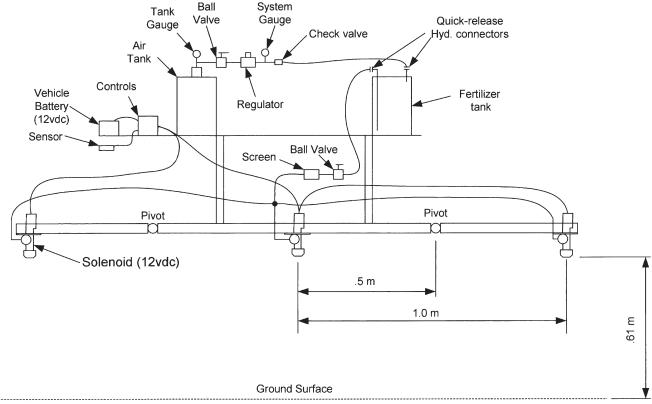
Fig. 5. Schematic diagram of the calibration stamp applicator retrofitted for assembly on a conventional four-wheeler including the air tank, fertilizer tank, electronics, and applicator boom.
