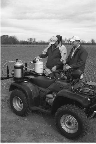
Fig. 2. Automated controller, 8-L pressured delivery tank, and onboard pressurized air tank.
