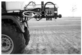
Fig. 4. Side view of the calibration stamp showing the outside nozzle and center three nozzles, and delivery of dyed urea ammonium nitrate via fan nozzles.
