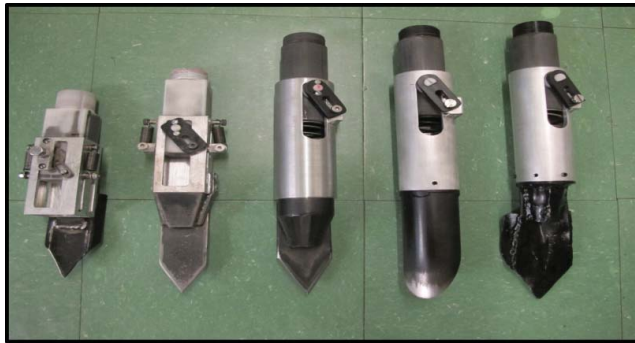
Figure 5. Sequential development (left to right) of the hand planter showing design progress and tip modification, 2011 through 2013.
