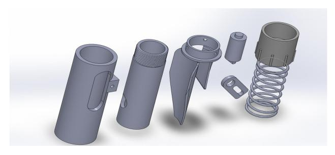
Figure 2: Components of seed metering unit (left to right), including external housing, internal housing planter trip, rotating drum, rotating arm, connecting coupler, and internal spring, Oklahoma State University.
