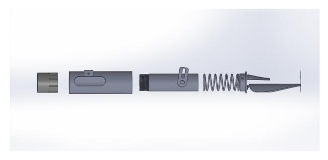
Figure 1: Side view of the maize hand planter showing (left to right) coupler, external housing, internal housing with rotating arm, spring and planter tip, developed at Oklahoma State University.
