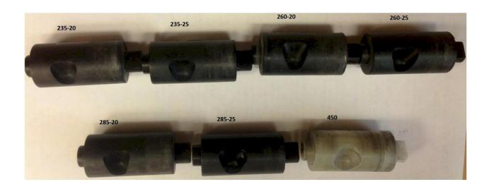
Figure 3: Internal rotating drums with different cavity depths, size, and angle.
