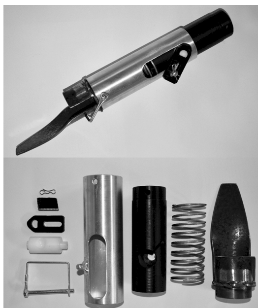
Fig. 2. Current 2018 hand planter and planter components developed primarily for maize producers in the developing world, who are entrusted with management on incredibly marginal landscapes.
