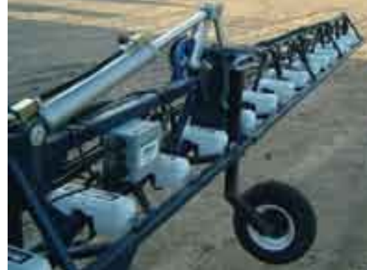
Consisting of a sensor and spray nozzle with fast-fire solenoid valve the WeedSeeker can accurately spot spray weeds reducing herbicide use and environmental impact.
