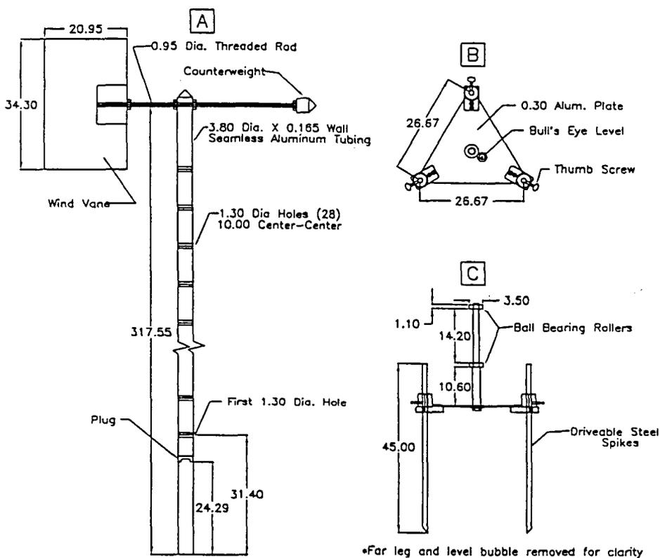
FIGURE 1. Schematic diagram of the rotating mast and base constructed for this study. (A) Side view of the rotating mast and windvane assembly. (B) Top view of the base. (C) Side view of the base. All numbers given are in centimeters.
