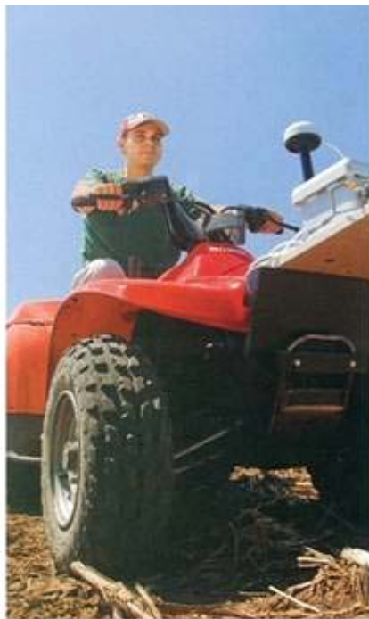
►Above: Crop canopy sensors designed to determine the nitrogen status of growing crops are being tested to map soil organic matter.
