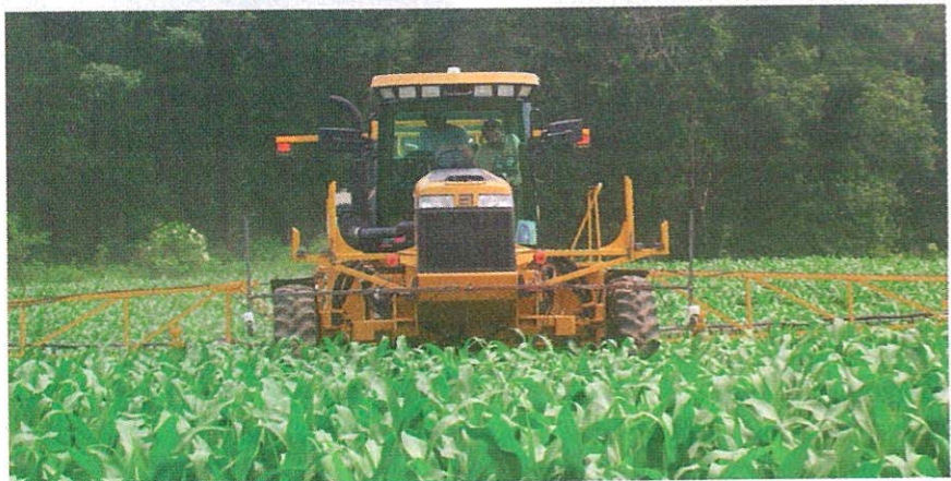
An 80-foot applicator from MFA Co-op in Mexico, Missouri, applied liquid N based on readings from two N sensors. Another dealer applied dry urea with a spreader truck.
