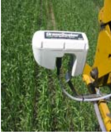
GreenSeeker RT200 on the go sensor reading wheat vigor.
