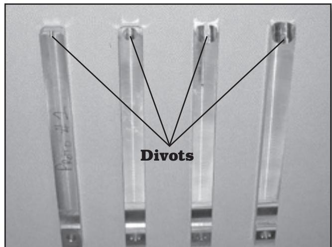
Figure 6–Different sizes of rams used for the Seed Stick. Each ram has a divot cut at its top to accommodate the seed. The ram must be changed for seeds of different sizes. The ram on the left was fabricated by the MTDC machine shop to accommodate tiny Douglas-fir seeds.
