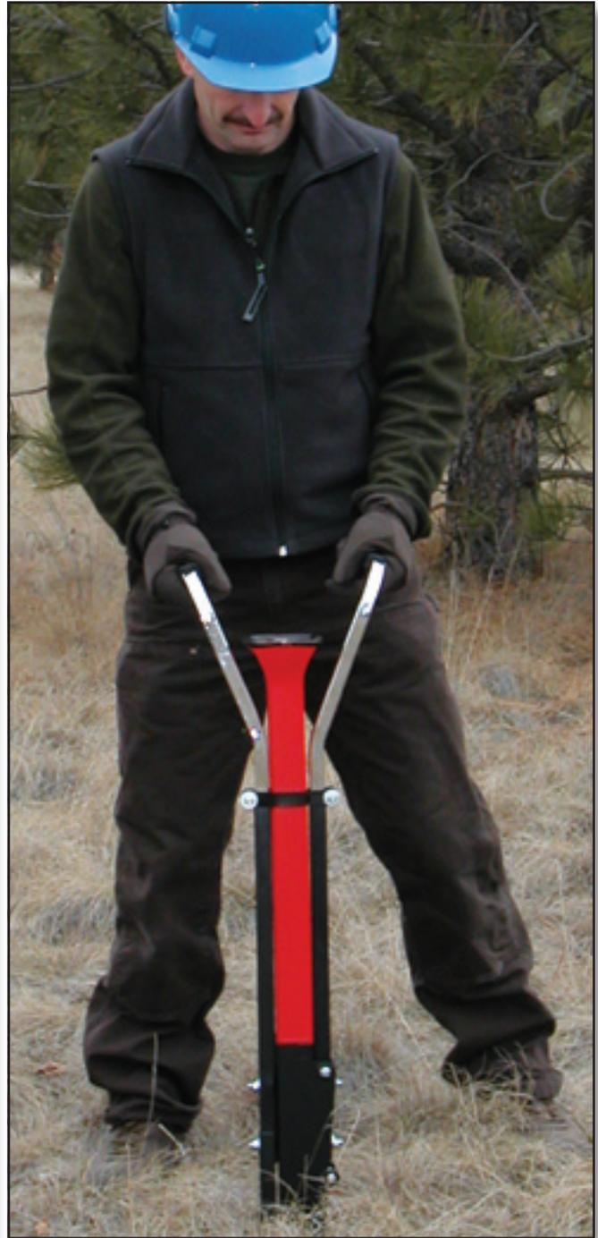
Figure 3—After the Hatfield Transplanter's bit penetrates the soil, the operator drops a seed, plug, or bulb into the hollow tube, and squeezes the planter's handles together, releasing the seed at the proper depth.
