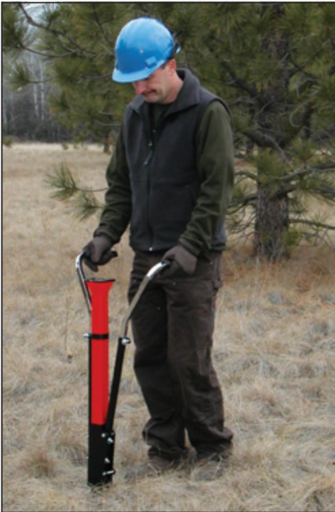
Figure 7—The Hatfield Transplanter was tested in a pine grove at MTDC.
