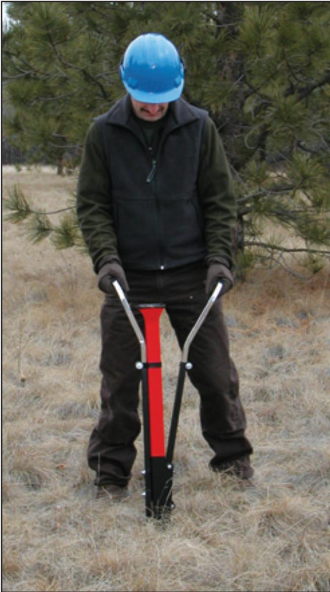
Figure 2—The Hatfield Transplanter's handles are open when the operator stabs the Hatfield Transplanter into the ground and steps on the foot plate.
