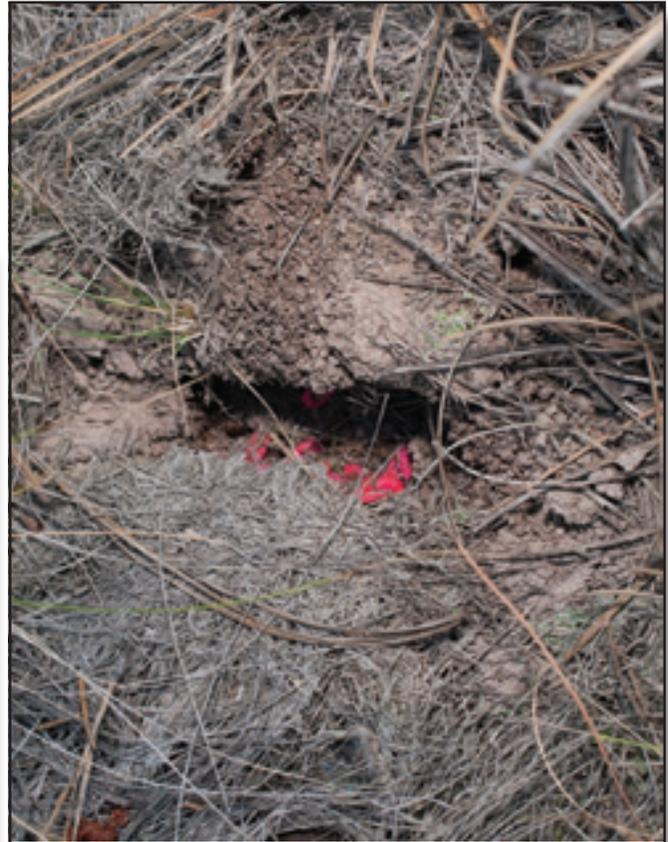
Figure 8—Whitebark pine seeds were painted red so they could be seen during testing. The seeds are shown in a hole made by the Almaco Hand Jab.
