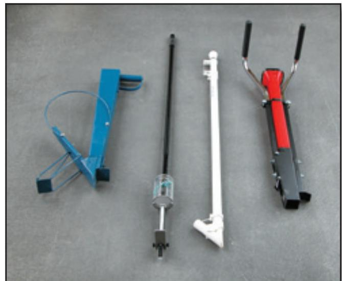
Figure 1—Planters tested were, from left to right, Almaco Hand Jab, Seed Stick, Stand 'n Plant, and Hatfield Transplanter.
