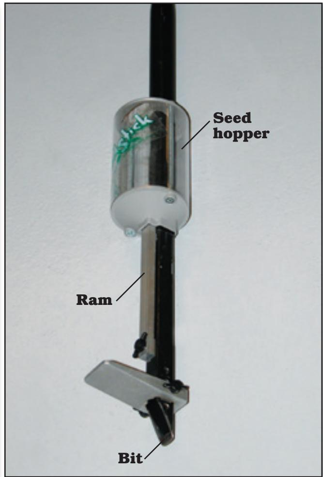
Figure 5–As the Seed Stick is pushed into the soil, a ram is pushed into the seed hopper, lifting a seed and dropping it into the hollow tube. When the operator makes a final push, the seed goes through the bit and into the soil.
