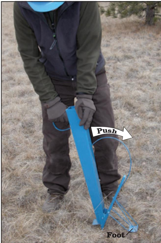
Figure 4–The operator stabs the Almaco Hand Jab into the ground and drops a seed into the hollow tube. To release the seed, the operator pushes the Almaco to the side on its “foot,” opening the bit.
