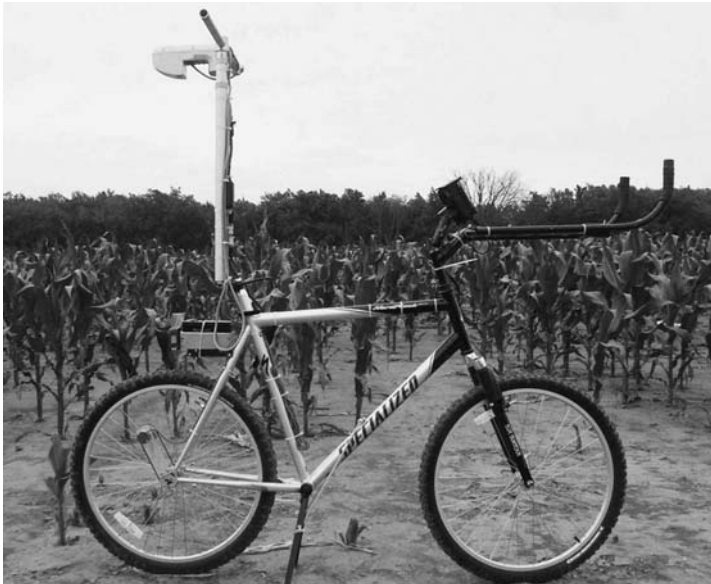
Figure 1. Framework for the bicycle and the adjustable pole that holds the sensor parallel and directly above the corn row. The shaft encoder is used to determine the distance at which NDVI is recorded is shown on the rear tyre of the bicycle.
