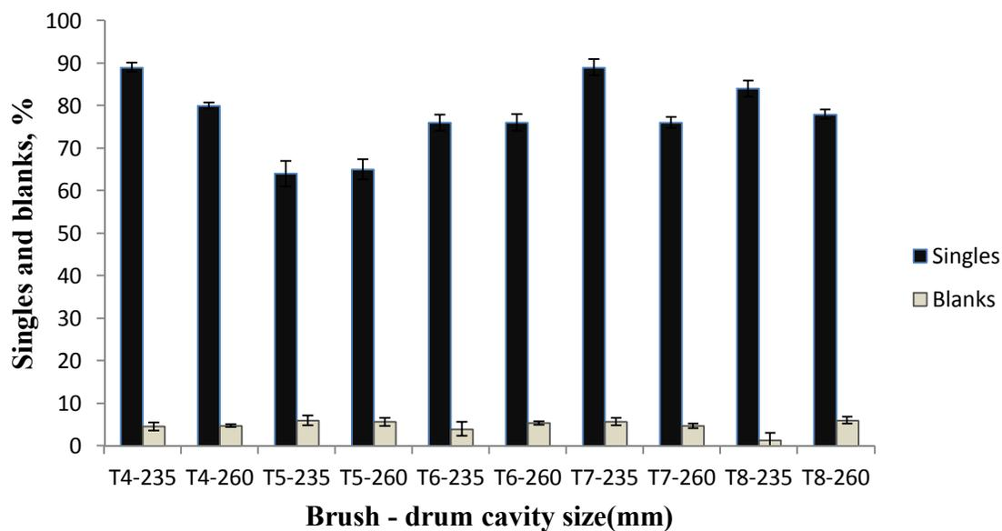
Figure 6: Distribution of maize singles and misses for brush and drum combinations averaged over 10 planter strikes (T-values represent different brush sizes and stiffness, 235 and 260 represent drum cavity depth in mm), September 2013.
