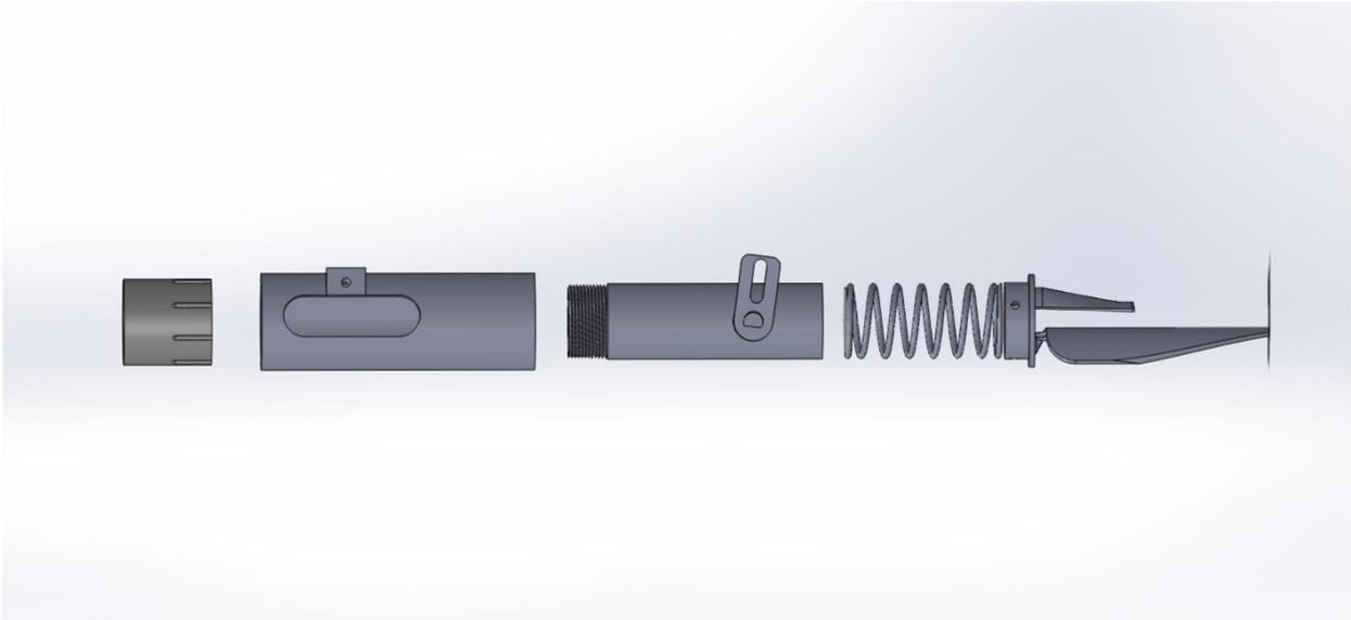
Figure 1: Side view of the maize hand planter showing (left to right) coupler, external housing, internal housing with rotating arm, spring and planter tip, developed at Oklahoma State University.
