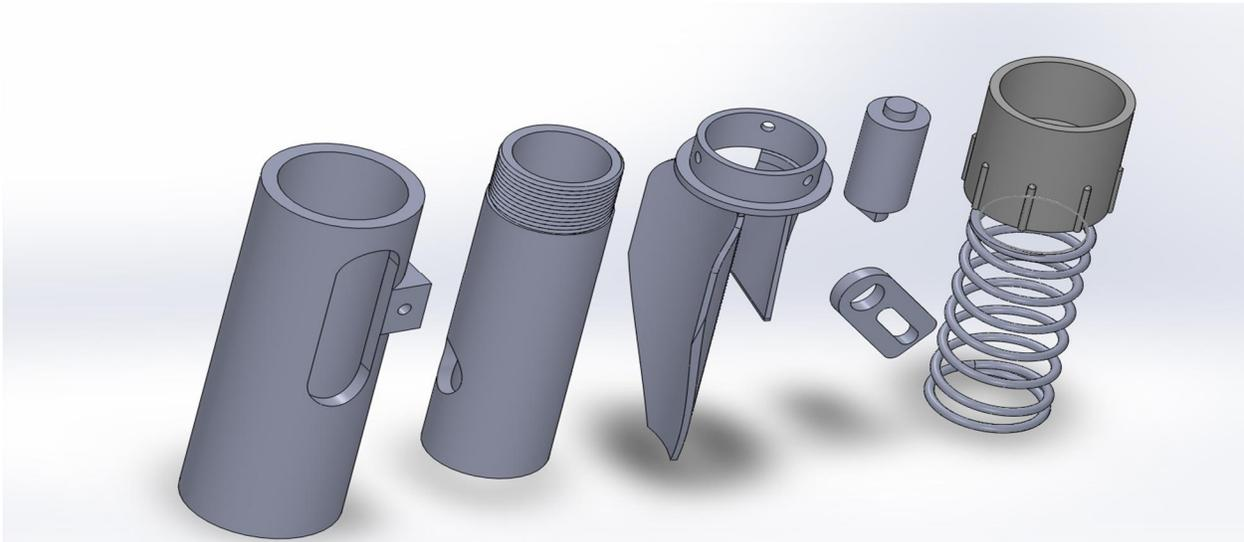
Figure 2: Components of seed metering unit (left to right), including external housing, internal housing planter trip, rotating drum, rotating arm, connecting coupler, and internal spring, Oklahoma State University.
