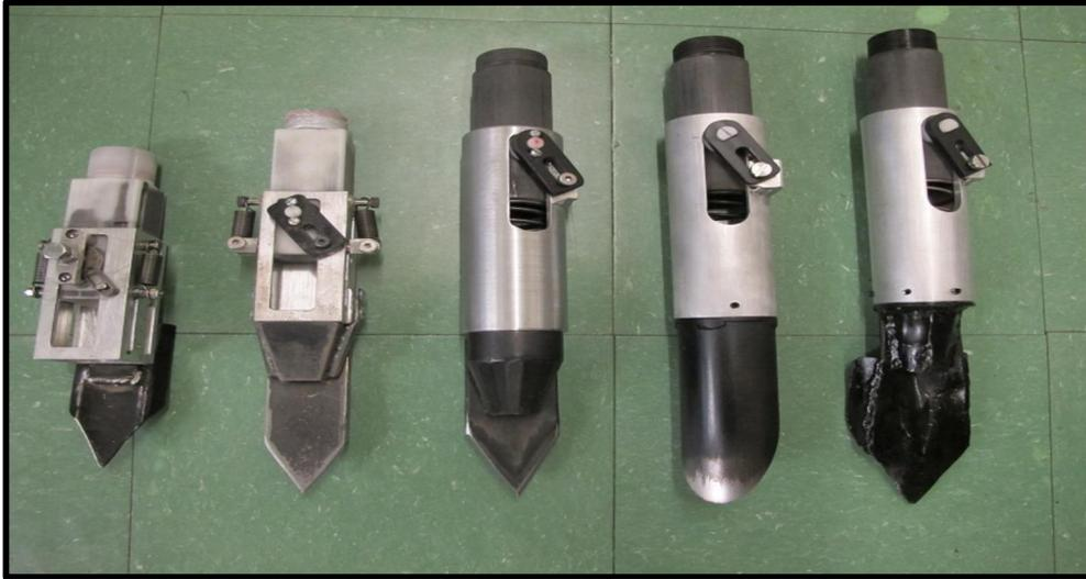
Figure 5: Sequential development (left to right) of the hand planter showing design progress and tip modification 2011 through 2013.
