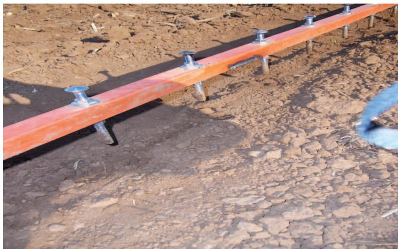
**FIGURE 2** Planting device constructed to establish fixed depths, and distances between plants for all sites, 2005–2006 (Color figure available online).
