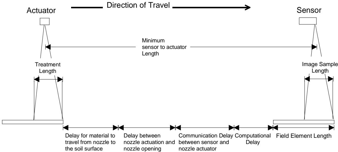
Figure 3. Factors affecting sensor to actuator distance
