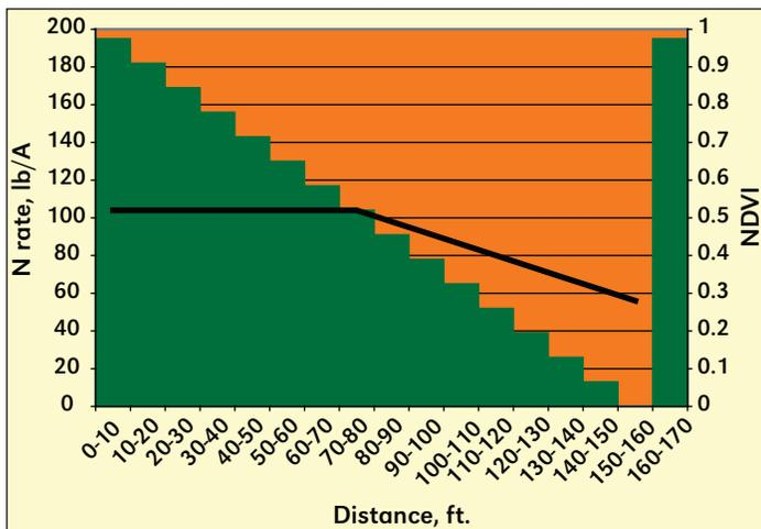
**Figure 1.** Fertilizer N applied and NDVI over distance traveled. Mid-season fertilizer N application is determined by finding the point where NDVI was maximized, then move horizontally to the desired N rate. In this wheat example from the EFAW Research Experiment Station located in Stillwater, Oklahoma, the optimal N rate in the spring of 2007 was 104 lb/A.
